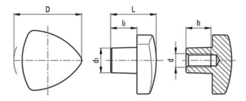
$\begin{array}{lll} D & = 50 \\ d & = M10 \\ d1 & = 18 \\ h & = 18 \\ L & = 33 \\ l2 & = 19 \\ Weight (g) = 150 \end{array}$
